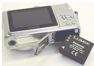
Figure 1 The digital camera shown here uses a rechargeable lithium-ion battery as its power source. These batteries are becoming the cell of choice for many portable electronic devices as they have a good shelf life and an exceptional energy density .
