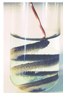
Figure 3 A copper coil placed into a silver nitrate solution quickly develops a thick silvery deposit of metallic silver as the colourless solution turns pale blue .
