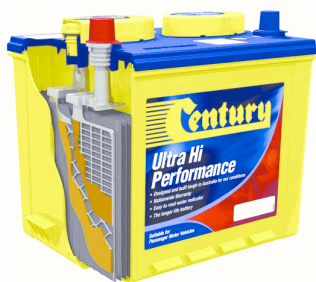
Figure 8 A typical car battery contains six lead-acid cells (Fig 9) connected in series in a single container producing 12 V.
