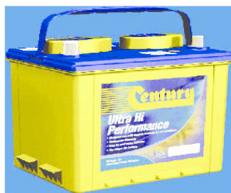
Figure 12 The basic technology of the lead-acid battery was first demonstrated to the French Academy of Sciences in 1860 by Gaston Planté. Each cell of a lead-acid battery has a lead-dioxide electrode and a spongy metallic lead electrode immersed in an electrolyte of 4.5 \text{ mol L}^{-1} sulfuric acid solution. Photograph courtesy of Century Yuasa Batteries Pty Ltd.
