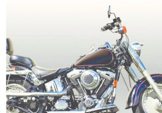
Figure 21 This Harley-Davidson motorcycle uses chrome-plating for corrosion protection and decorative effects.
