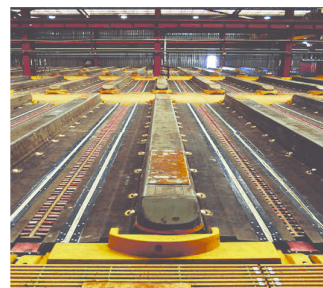
Figure 24 The pure and impure copper electrodes of a commercial electrorefining plant are shown here. The electrodes are suspended in a copper(II) sulfate electrolyte. A potential difference applied to the electrodes causes impure copper to dissolve while pure copper is deposited at the cathode. Below you can see stacks of 99.99% pure copper cathodes ready for export.
