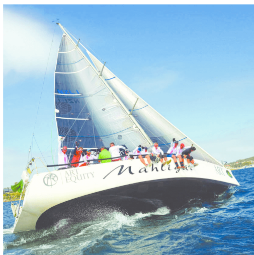
Figure 8 The strength, durability and low density of many polymers is used to great advantage in sail boat construction. Here they have application in sail making and as a composite material (two or more materials bonded together) in hulls and superstructures.
