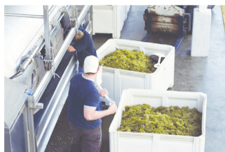
Figure 11 Chardonnay grapes being prepared for crushing. Before fermentation the grape mixture of juice, skins and seeds, called must , should have a pH of around 3.5 or less. If pH is too high, tartaric acid (a white crystalline diprotic acid \text{C}_4\text{H}_6\text{O}_6 ) is added to increase its acidity. If pH is too low then potassium bicarbonate ( \text{KHCO}_3 ) can be added to make it more alkaline.
