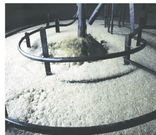
Figure 6 Fermenting sugar from sugar cane produces ethanol. Notice the foaming surface. This is due to the formation of \text{CO}_2(\text{g}) .
