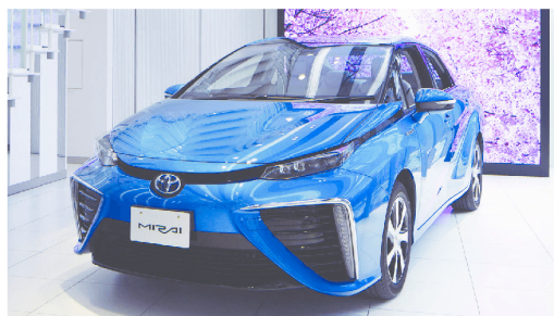
Figure 15 This Toyota Fuel Cell Vehicle (FCV) is scheduled for selected release into the Japanese car market in early 2015 prior to its release in the US and Europe. It utilises solid polymer electrolyte membrane fuel cells (similar to the PEMFC) and a nickel metal hydride storage battery to power its electric motor. Hydrogen is stored at 70 MPa in several storage cylinders giving the vehicle a range of around 700 km.
