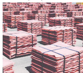
Figure 24 The pure and impure copper electrodes of a commercial electrorefining plant are shown here. The electrodes are suspended in a copper(II) sulfate electrolyte. A potential difference applied to the electrodes causes impure copper to dissolve while pure copper is deposited at the cathode. Below you can see stacks of 99.99% pure copper cathodes ready for export.
