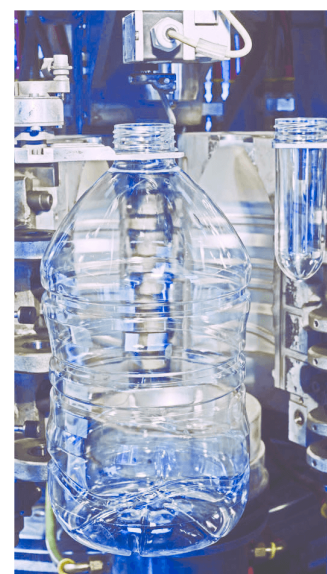
Figure 5 A PET drink bottle being formed in a stretch blow moulding machine. Note the initial shape of the 'preform' bottle at the top right.
