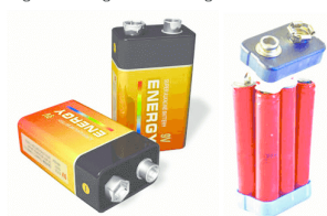
Figure 1 Galvanic cells like the dry cell are typically referred to as batteries. Specifically though, a battery is a group of two or more galvanic cells, usually connected in series (terminals connected + to -), to produce a higher voltage than a single cell would.
