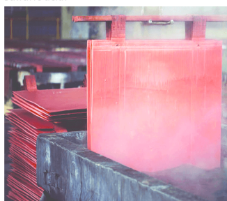
Figure 18 Pure copper cathodes being removed from an electrolyte bath of copper(II) sulfate dissolved in dilute sulfuric acid.
