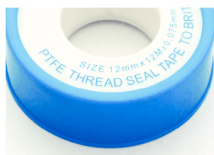
Figure 4 Plumbers apply a thin layer of PTFE tape to threaded connections. The PTFE film prevents the join from becoming chemically fused and helps form a watertight seal.
