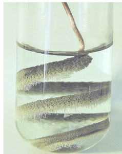
Figure 16 Silver depositing on a copper coil. 2\text{Ag}^+(\text{aq}) + \text{Cu}(\text{s}) \rightarrow \text{Cu}^{2+}(\text{aq}) + 2\text{Ag}(\text{s})
